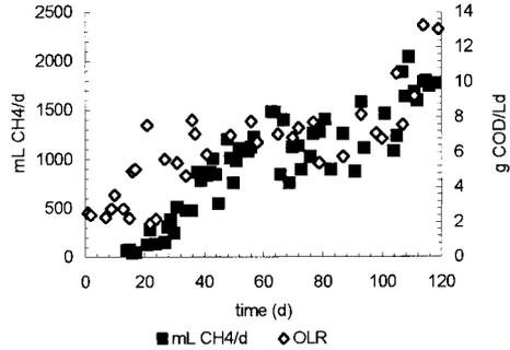
Figure 7 Performance of methane production and OLR
