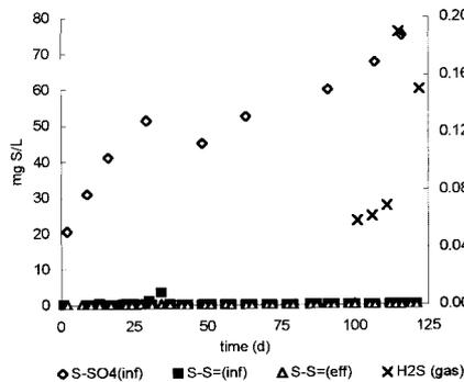
Figure 8 Sulfur species in liquid and gas phase
