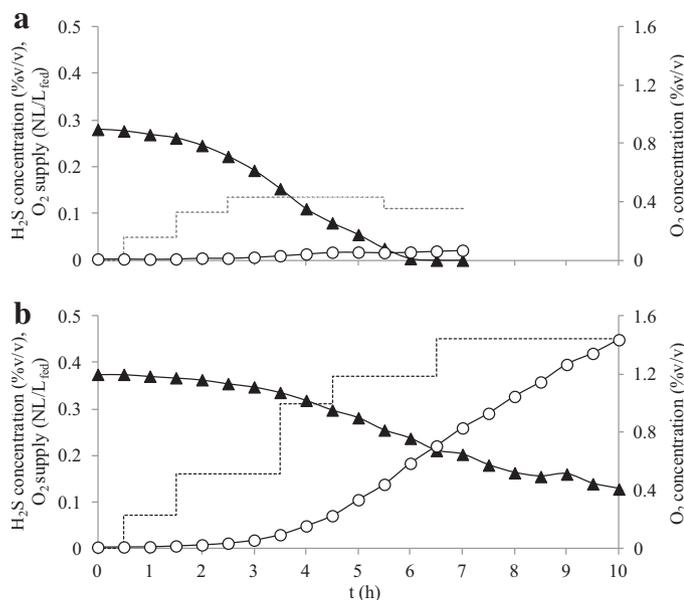
**Fig. 4.** O<sub>2</sub> flow rate (discontinuous line), and concentrations of H<sub>2</sub>S (▲) and O<sub>2</sub> (○) in the biogas from R1 and R2 at  $t = 16$ .
