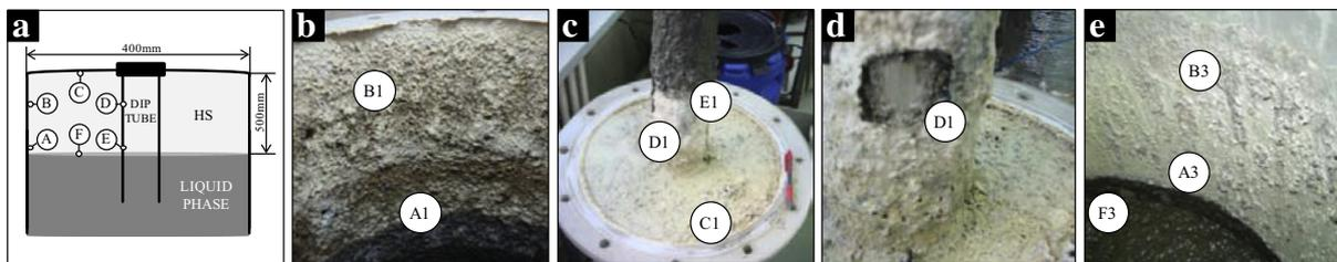
Fig. 3. HS diagram and samples codes (a). Walls of the HS (b), ceiling and dip tube (c and d) of R1 at  $t = 15$ . Walls of the HS and liquid interface of R2 at  $t = 17$  (e).
