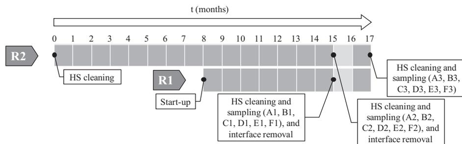
Fig. 2. Operational sequence. ▨ : microaerobic period; ■ : anaerobic period.
