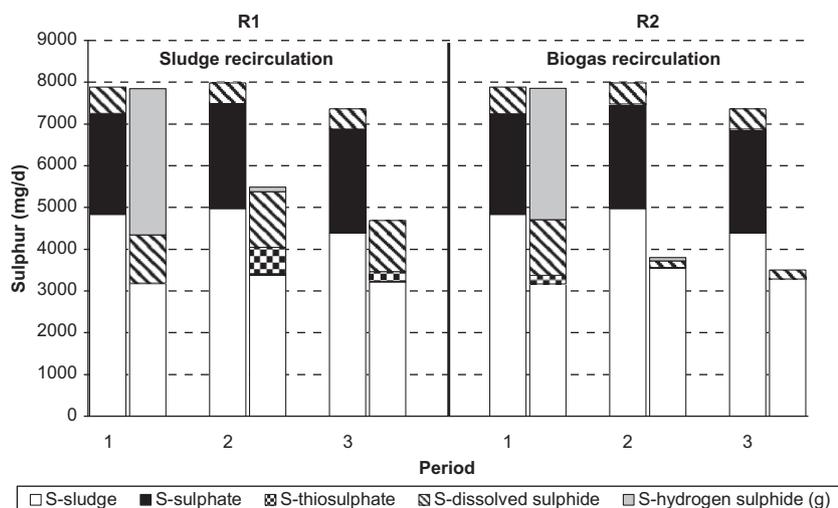
Fig. 3. Sulphur balance during the study. For each period, left column: inputs; right column: outputs.
