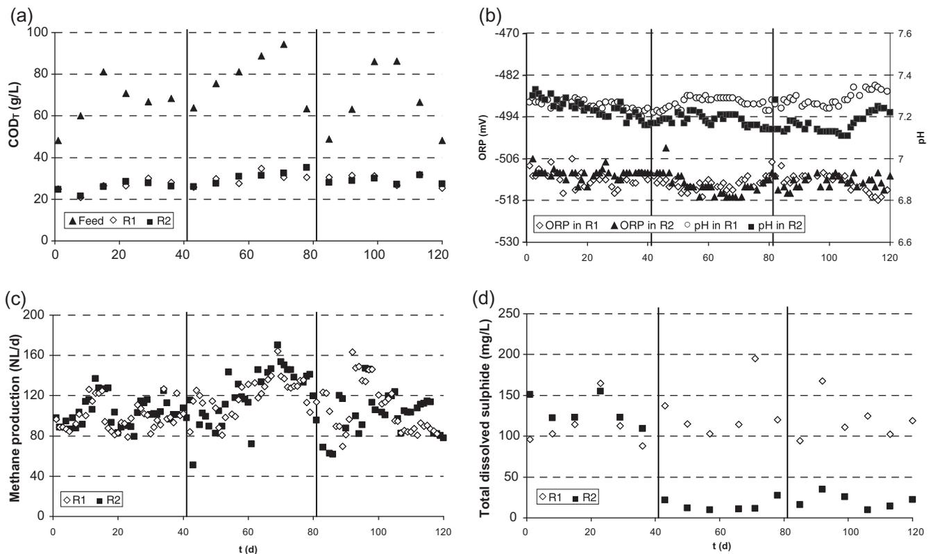
Fig. 5. Digestion behaviour during the study. (5a) COD<sub>T</sub> in feed and digested sludge. (5b) ORP and pH in digesters. (5c) Methane production. (5d) Total dissolved sulphide concentration in digesters.
