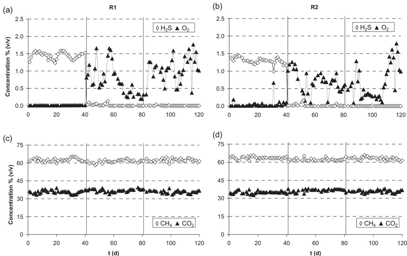
**Fig. 2.** Biogas composition in %(v/v). (2a) Hydrogen sulphide and oxygen concentrations in R1; (2b) hydrogen sulphide and oxygen concentrations in R2; (2c) methane and carbon dioxide concentrations in R1; and (2d) methane and carbon dioxide concentrations in R2.
