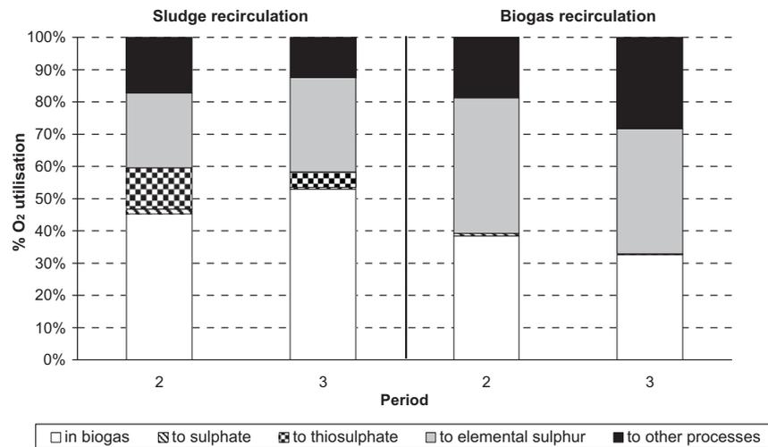
Fig. 4. Estimated oxygen utilisation in digesters.
