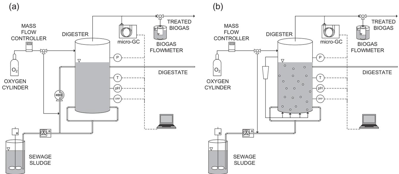
Fig. 1. Pilot-plant diagram. (1a) Reactor 1 (sludge recirculation) and (1b) Reactor 2 (biogas recirculation).
