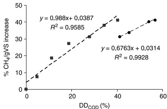
Figure 6 | Biogas production vs. disintegration degree for tests A (■) and B (●).
