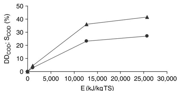
**Figure 1** | Solubilisation (●) and disintegration degree (▲) vs. energy, for 200 W and different sonication time.
