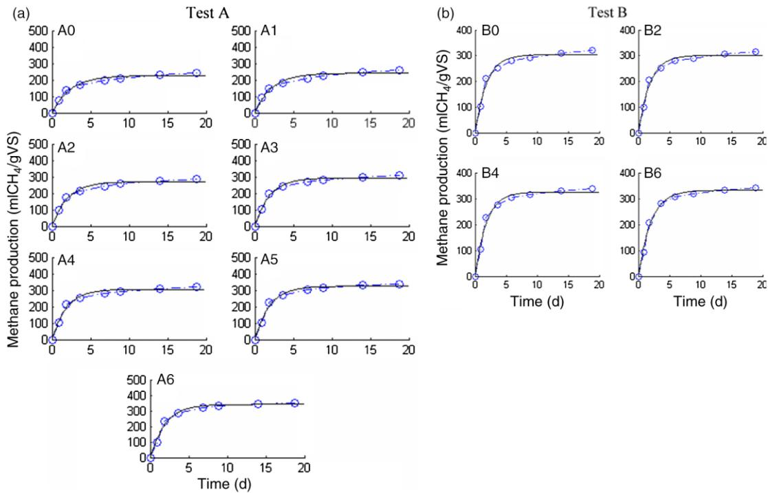
**Figure 3** | Model fit to experimental data of biogas production for tests A and B.
