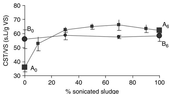
Figure 9 | CST vs. % sonicated sludge for digested sludge from tests A (■) and B (●).
