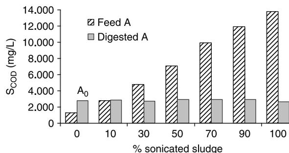
Figure 7 | SCOD for sludge feeds and digested sludge from tests A.
