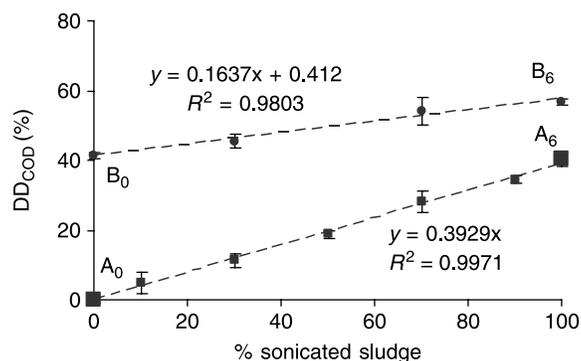
**Figure 2** | Disintegration degree vs. % sonicated sludge of sludge feed for tests A (■) and B (●).
