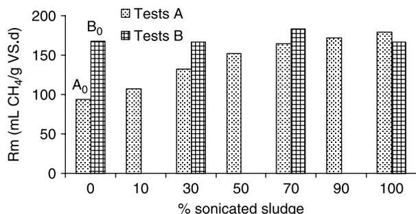
Figure 5 | Maximum biogas production rates from kinetic model fit for tests A and B.
