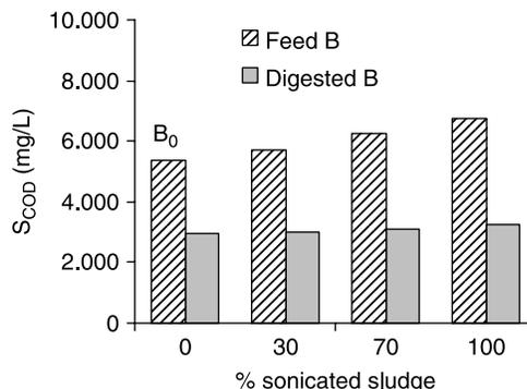
Figure 8 | SCOD for sludge feeds and digested sludge from tests B.
