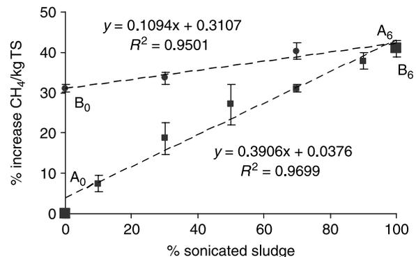
**Figure 4** | % increase of L CH<sub>4</sub>/kg TS vs. % sonicated sludge for tests A (■) and B (●).
